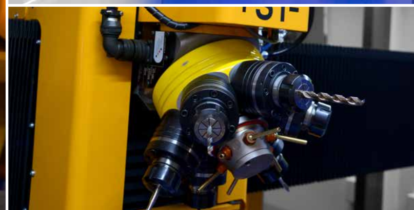
Turret drilling head with 6 tool positions for drilling up to Ø 20 mm and tapping up to M16
