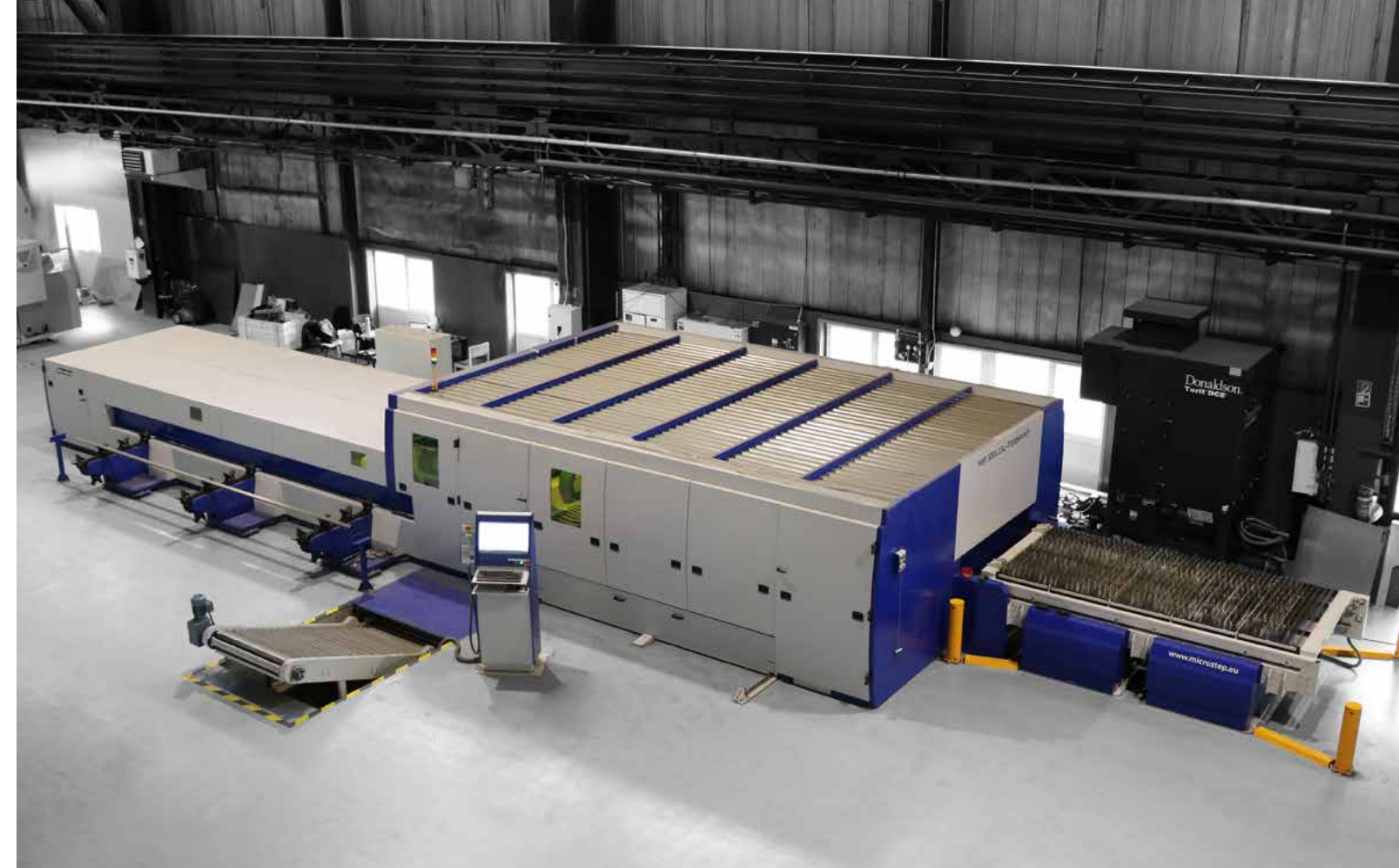
A versatile CNC fiber laser cutting machine for sheets and pipes with laser power up to 10 kW
